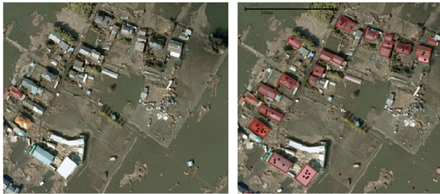
Fig. 10 Left is northwest corner of satellite photo in Fig. 9, and right is the same area after build-out using DroneLab environment builder. Buildings shown as red rectangles and survivors as red dots. Photograph by GSI of Japan (Geospatial Information Authority of Japan 2011)
