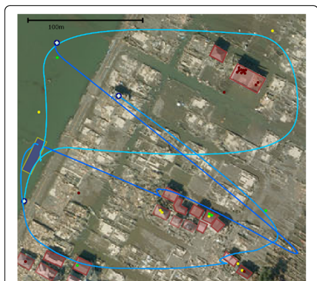
Fig. 7 Scatter method showing the paths of three UAVs. As with standard method, robots launched from the blue rectangle. However, each UAV proceeded to a different location in the search pattern, scattering them across the area. Photograph by GSI of Japan (Geospatial Information Authority of Japan 2011)
